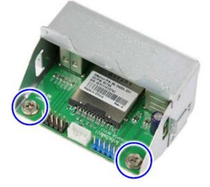
8. Remove the front I/O and card reader assembly from the bracket.
